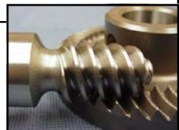
Complete assembly and machine manufacturing, such as the ITW Hi-Cone beverage packaging machine, is shown above. Shown in the inset: a Precision Spiroid® gearing.
